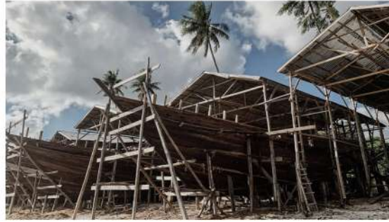
Phinisi in build at the beach – the construction techniques have barely changed over the centuries
